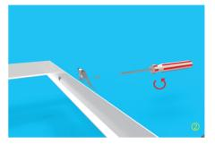
2.Installing the frames. Putting one side of the frames into ceiling hole and fixing it with spring clips, following the way to fix another side, ensuring the frames fixing wall and safe, putting the panel light fixture inside and place it on the recessed frames.
